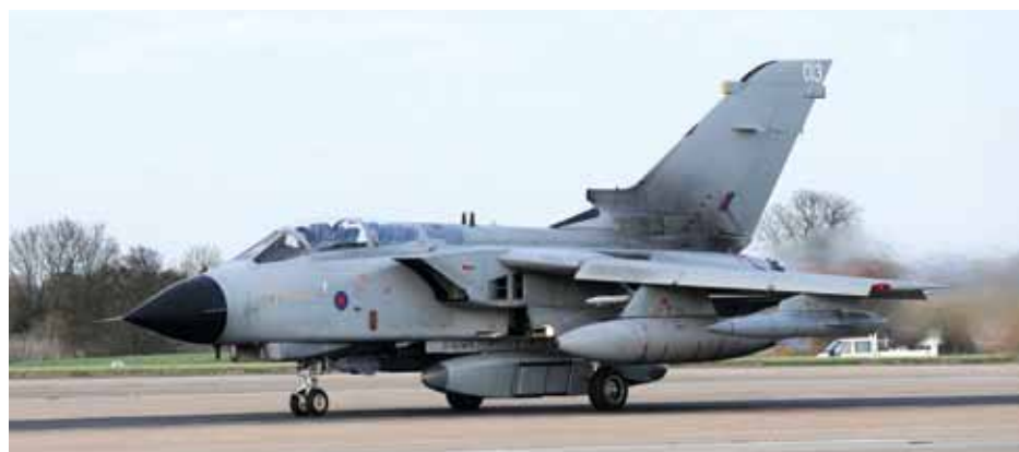
Above: The bulky RAPTOR pod considerably reduces ground clearance on the Tornado, the main reason it can't be used on Typhoon. Crown copyright/MoD
