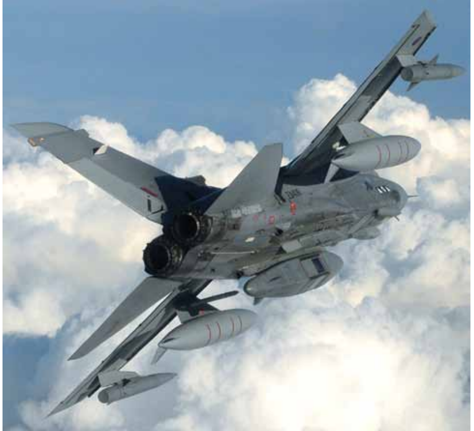
Above: The RAPTOR pod is seen to advantage on this shot of Tornado GR4 ZA406 with 'Shiny Two' Squadron nose bars. The pod is carried on the left-hand under-fuselage stores station. Peter R Foster
