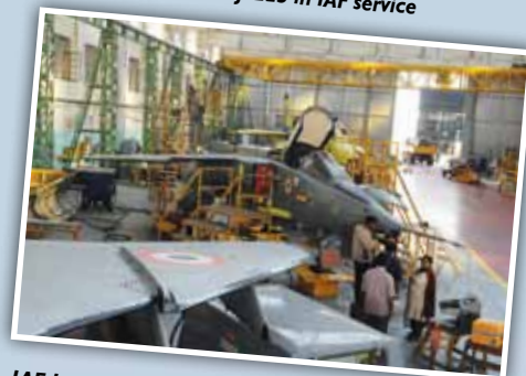
IAF Jaguars undergoing servicing in the hangar
